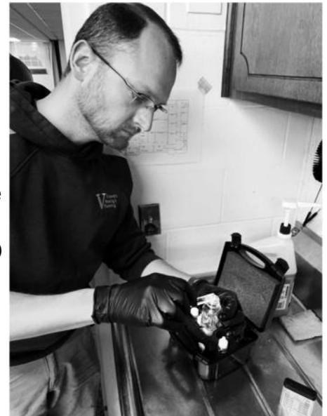
Here is Marvin performing a water test for a customer on a recent job. Water quality - especially hardness - affects the function of your plumbing fixtures - and can have negative health impacts.
